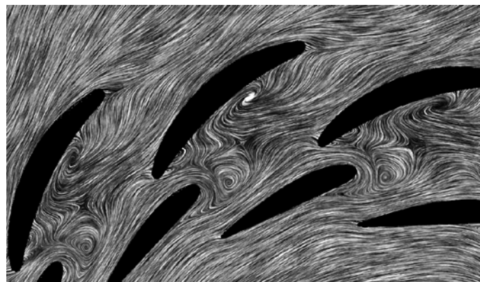
Fig. 2.9: Line Integral Convolution (LIC) image of 2D flow in the stator of a pump-turbine in pump mode (reversed); main flow direction is from lower left to upper right.
